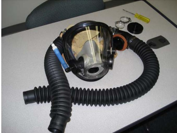
2. Remove the breathing chamber lid, PCM, and three moisture control sponges from the BioPak 240R. Wash and rinse the chamber lid, PCM and moisture control sponges. **RINSE THOROUGHLY!** Make sure you squeeze out the excess water from the moisture control sponges after both the wash and rinse cycle. Set the moisture control sponges on a clean surface and allow to **air dry in a dust free environment.**
